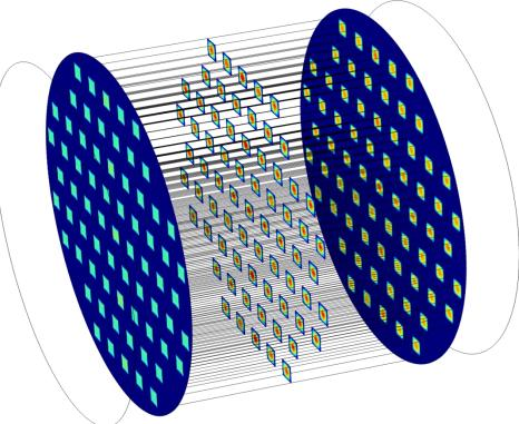
Quarter of full geometry of monolith (with 69 rectangular square channels with sides of 2 mm and length of 1 m)
