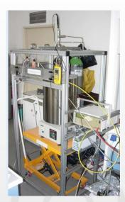
Experimental unit for high temperature CO<sub>2</sub> sorption (UCT)
