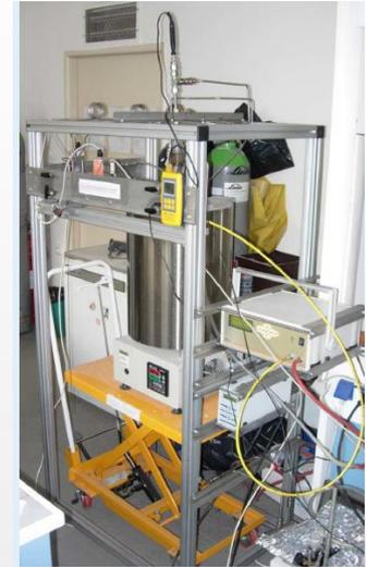
Experimental unit for high temperature CO<sub>2</sub> sorption (UCT)
