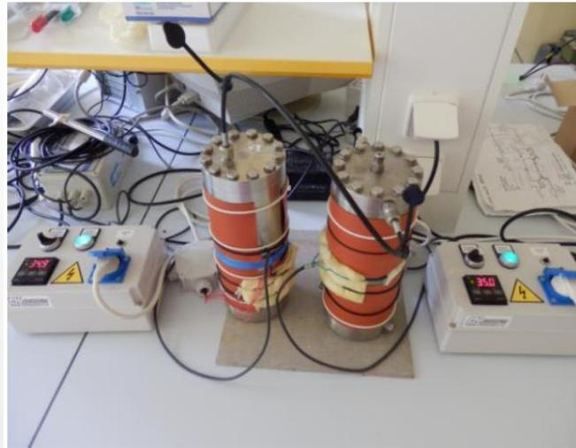
Photo of the apparatus used for long-term static experiments - REPP-CO<sub>2</sub> (UJV, CGS)
